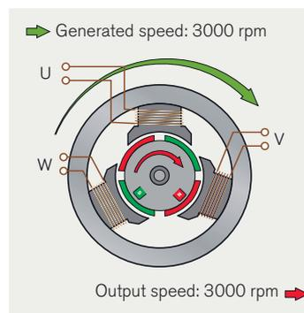
In a synchronous motor, the rotor rotates at the same rate as the stator field per the electrical frequency.
