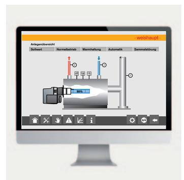
An optional analogue or bus expansion module makes the remote operation, diagnosis, and monitoring of the burner possible.
