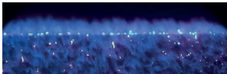
*The homogeneous mixture of gas and air combusts on the surface of the woven metal mesh at temperatures < 1200 °C. This combustion technology effectively inhibits the formation of thermal NO<sub>x</sub>.*
