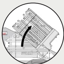
Mixing assembly in servicing position
