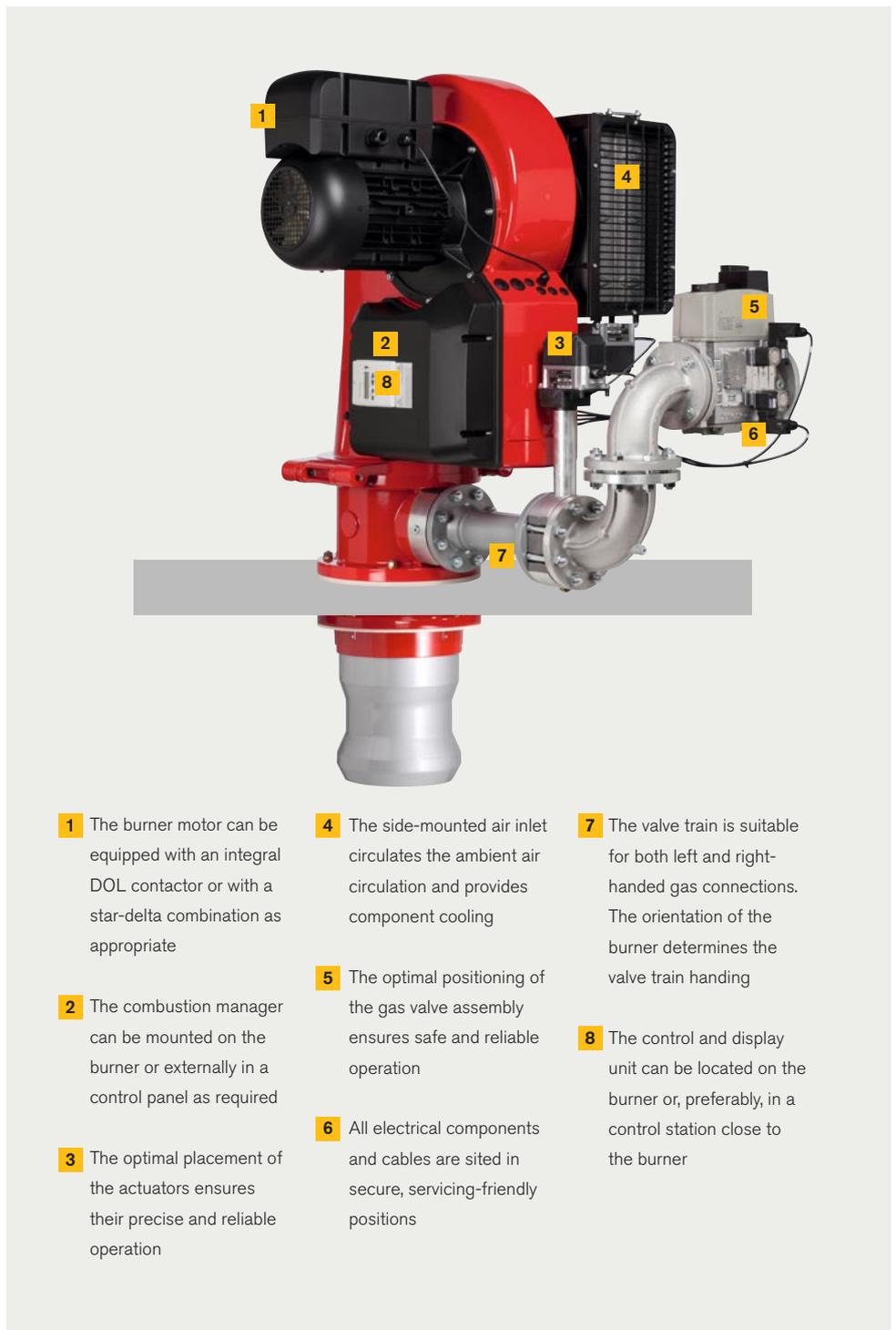
**1** The burner motor can be equipped with an integral DOL contactor or with a star-delta combination as appropriate
